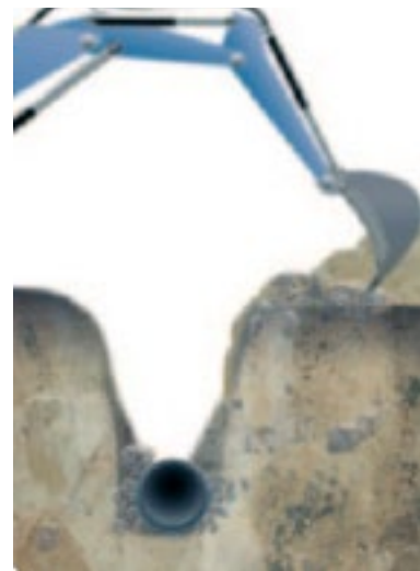
Fig 2-3: When installation is not executed in a sandbed, pipes with integrated protective layers are recommended to be used.
