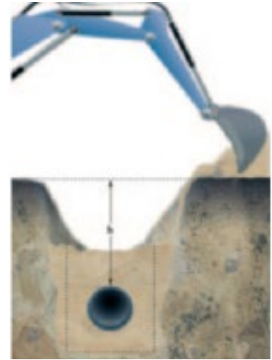
Fig 2-2: Standard pipes are installed in a sand bed
